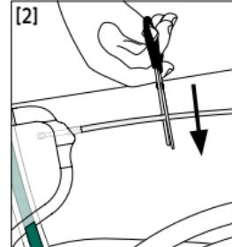
Use scissors to cut the inlet tube to the desired length (left: angled cut with a hard tube, right: straight cut with a soft tube).
